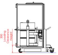
The drum mixer is designed to interface with our DTPO4 to provide a safe and easy way to load and unload the drum mixer. The image below shows the easiest way to load the DMEO1 which is using our DTPO4 Side-Shift Drum Depalletiser.
